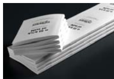
Multiple stitching allows 2-up or 3-up production
